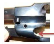
5. Once assembled if the lip is not in front of the cylinder pin (Fig.4), you will need to remove material from the bottom of the 1858 Remington Cylinder Pin Quick Release. Remove material slowly because if too much material is removed the plunger and spring will drop out.
