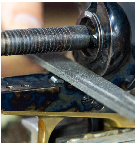
Fig. 9 File used to create flat pads for the feet
